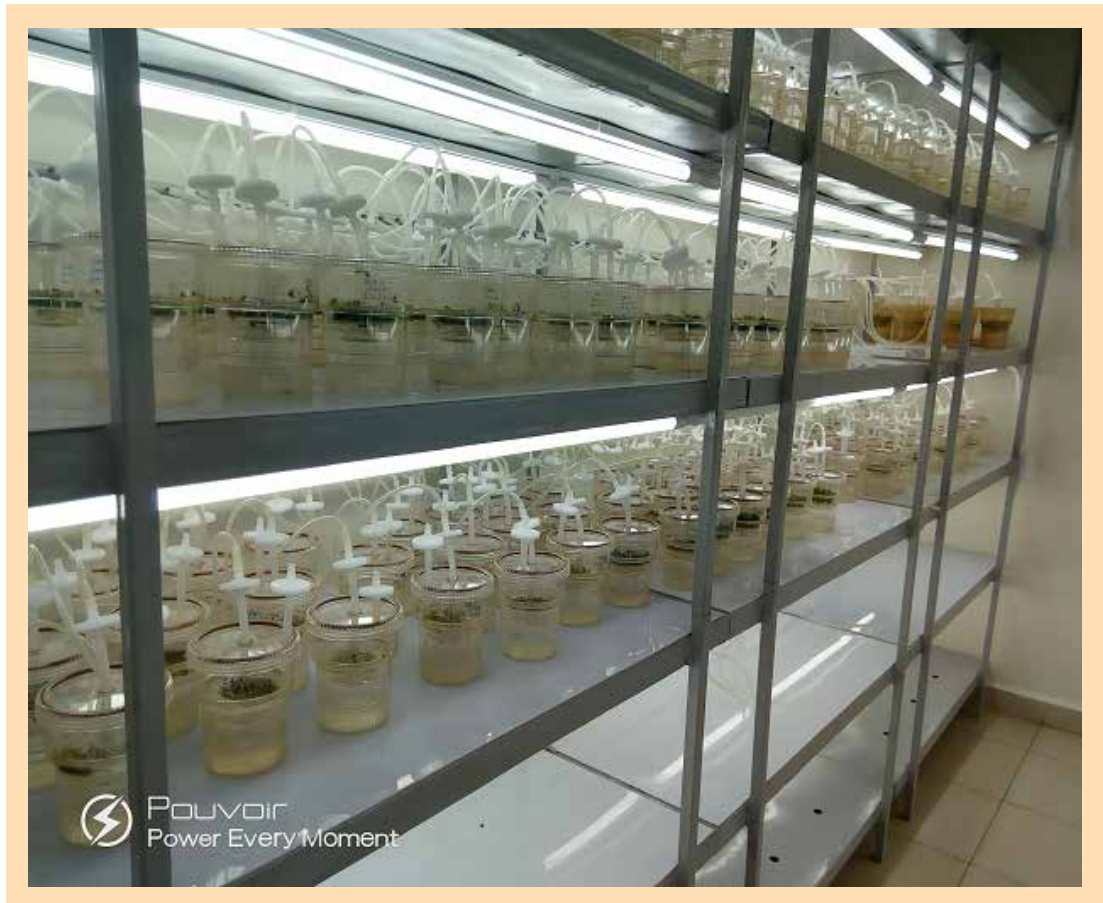
Figure 22: New RITA bio-reactors deployed in the biotechnology laboratory
